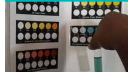
pH value, ammonia, iron, nitrate & phosphate testing based on colour indication.
